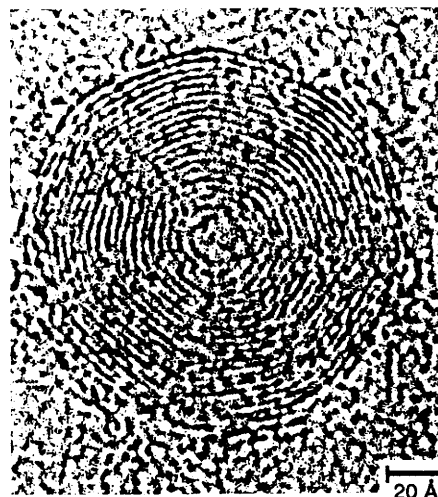
Fig. 3 Transmission electron microscope image of a spheroidal graphite microparticle observed by Iijima 20 in 1980
